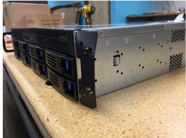
Server damage (bent case)
