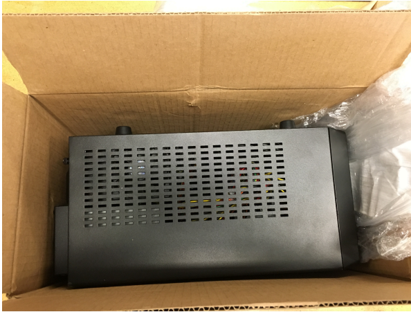
Server shipped in single-wall box with NO padding
