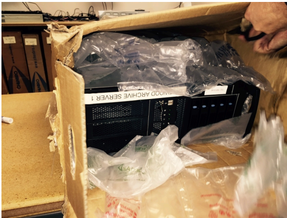
Server shipped in used single-wall box with insufficient padding (air bags)
