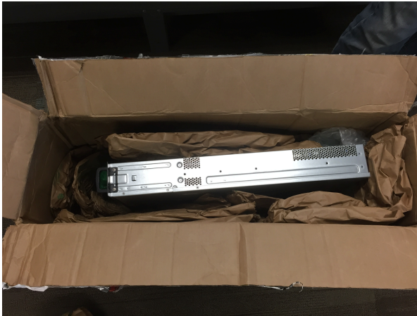
Server shipped in used single-wall box with insufficient padding (kraft paper, bubble wrap)
