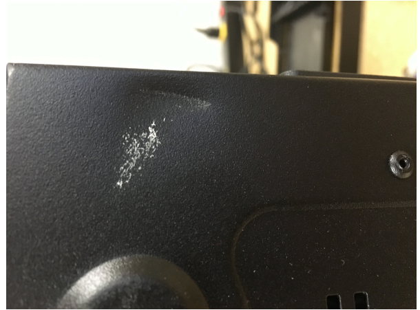
Case dented, face plate damaged, and server feet broken off
